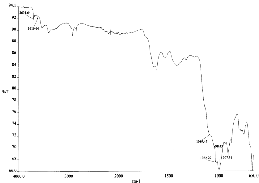
Figure 8. Infrared spectrum of gold and red paint from cloak. Gold/red side was against the ATR element.
