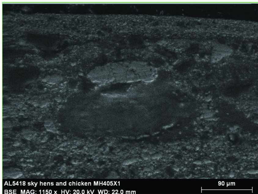
Figure 11. 1150 \times magnification. SEM-BSE image (uncoated sample analyzed using variable pressure mode) of a lead soap aggregate in the imprimatura layer; the aggregate is the large dark oval-shaped area at the center of the image (Sample 405 x01).
